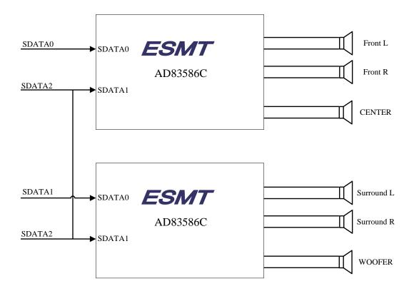
The AD83586C allows designers to achieve reliable, high-power audio, with up to 96-kHz flexible processing and self-protection features including short circuit, over-temperature protection and DC speaker protection.
